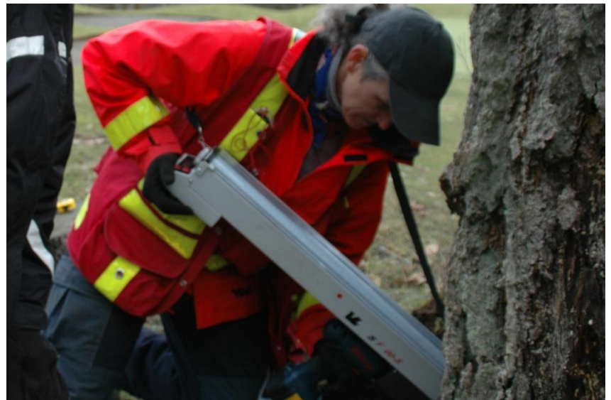
Verna Mumby using a Resistograph 2 to confirm the presence of decay in a large Douglas fir tree.
